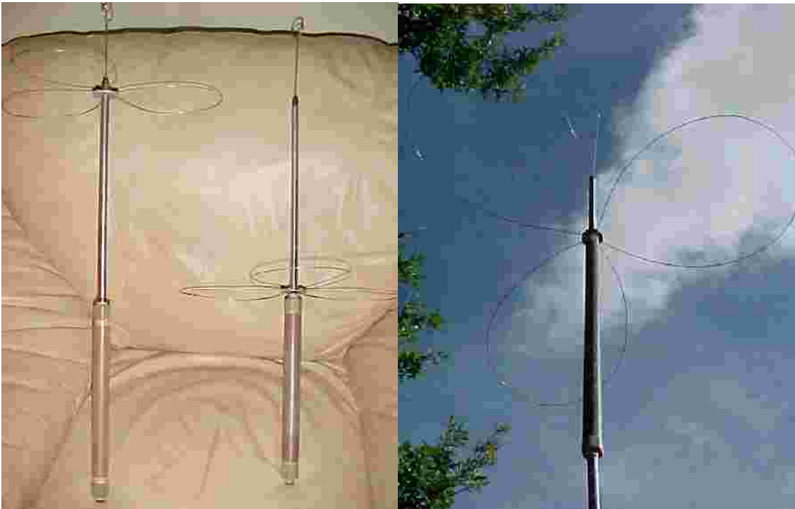
Figure 35. An 3.8MHz resonator with HI & LO hats. Figure 36. A 1.8MHz resonator with a low hat
