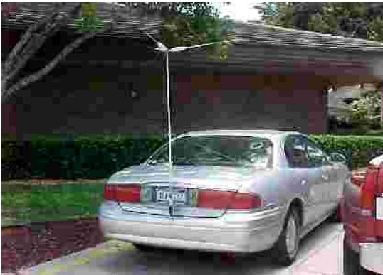
Figure 1. Typical mobile antenna with multiple resonators
