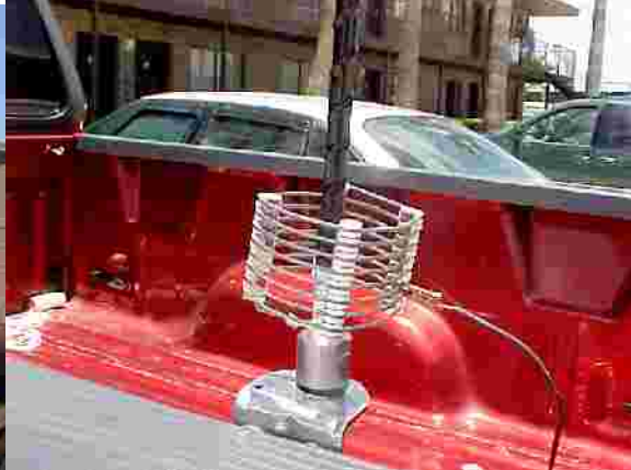
Figure 42. A small commercial “screwdriver” antenna. Figure 43. Shunt matching coil at the base of an antenna.
