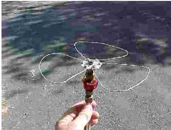
Figure 38. 14.2 MHz toroidal resonator.
