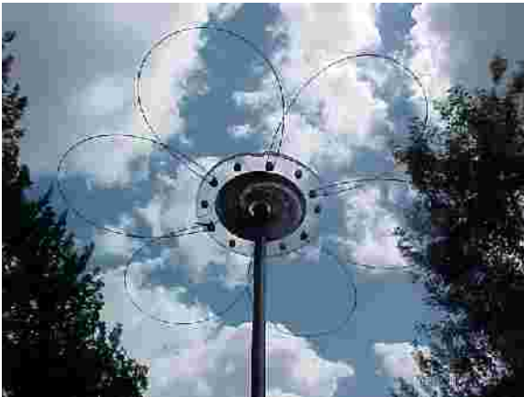
Figure 37. 3.8 MHz pie-wound resonator on a 1/2" mast.
