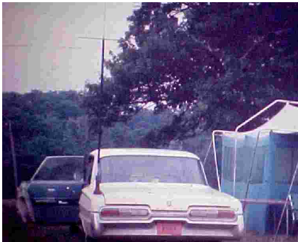
Figure 8. The modified "Bandspanner" using a tank mount and spring from WW2
