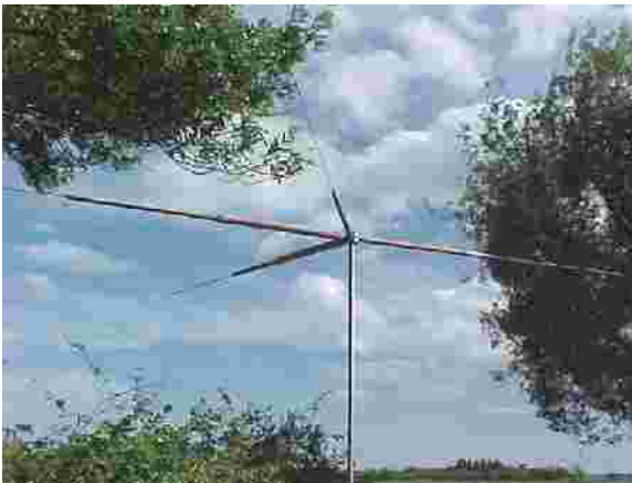
Figure 29. Multi-resonator setup with 40, 30, 20 & 15 meters in place.
