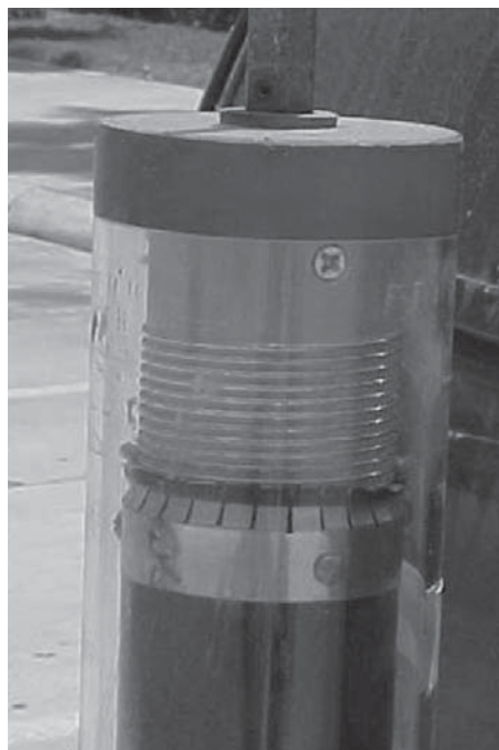
Figure 40 —The coil used to resonate the antenna on 20 m.
