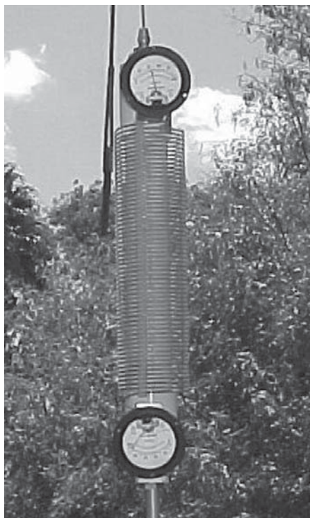
Figure 42 — RF ammeters reading 100 mA on the bottom and 42 mA on the top of the loading coil.
