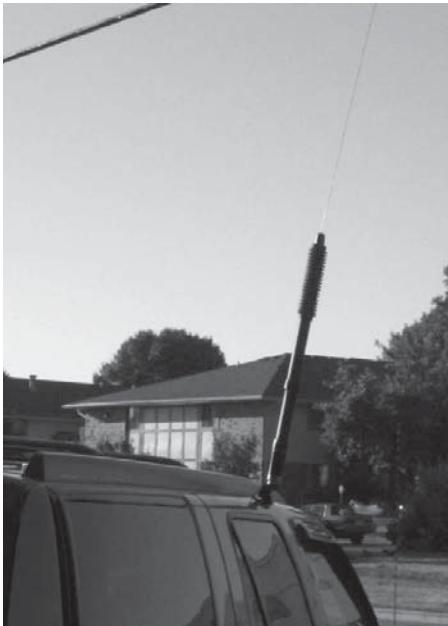
Figure 36 — A small commercial "screwdriver" antenna.
