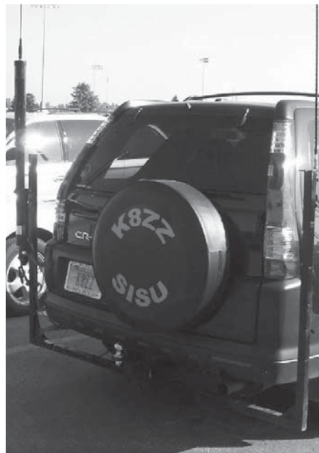
Figure 39 — Note the parallel beam mounting structure.
