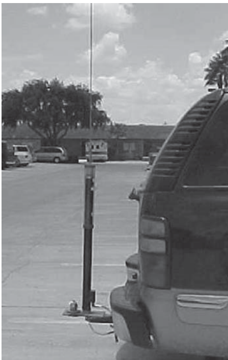
Figure 38 — A large commercial "screwdriver" motorized antenna.
